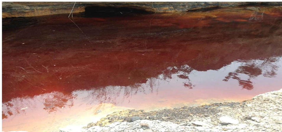
Figure 2. Precipitation of ferric iron as hydrated iron oxide.
