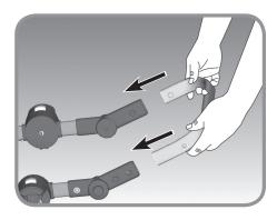
**3** Insert Foot Bar from the Bassinet Kit into the seat frame until it clicks into place.
