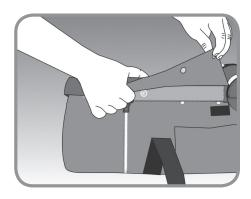
**6** Fasten all snaps around the top portion of the Bassinet to the top portion of the seat frame.
