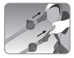
**2** Remove footwell frame from upper seat frame by pressing buttons on both sides of footwell and gently pulling until the pieces separate.
