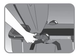
**9** Unzip mesh canopy fabric and set aside. Snap canopy brackets to both sides of seat frame.
