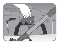
**13** Align Bassinet bracket adaptors with mounting brackets on your stroller. Press firmly until bassinet clicks into place.
