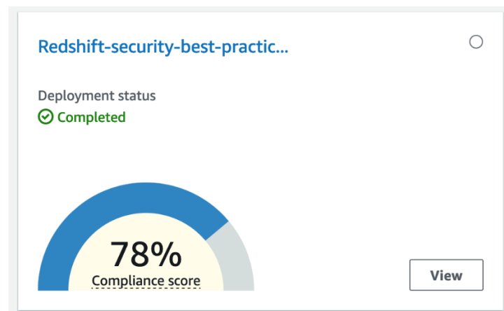
Figure 11 – The percentage of passing rule-resource combinations can be tracked to give an indication to overall conformance across your clusters.
