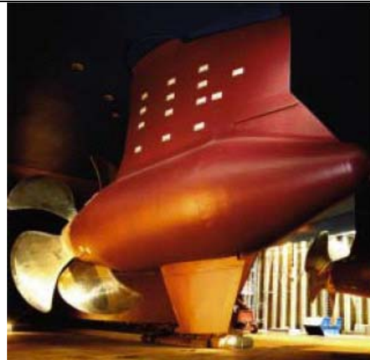
b) Radiance of the Seas , 2 x 19,5 MW Azipod® propulsion – ABB Marine
