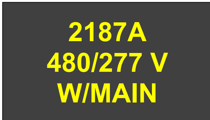
Figure 15. Distribution panel with main power source entry plate/label; 7/8-inch-high yellow letters on 4-inch high by 7-inch-wide black background (figure is approximately 1/2 scale)
