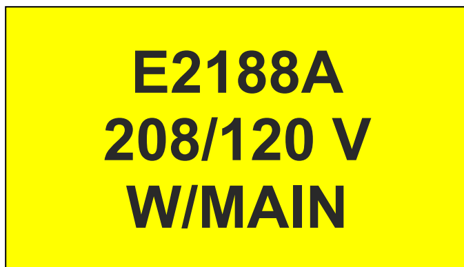
Figure 16. Distribution panel with main emergency power source entry plate/label; 7/8-inch-high black letters on 4-inch-high by 7-inch-wide yellow background (figure is approximately 1/2 scale)
