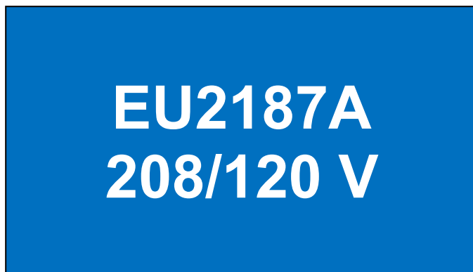
Figure 18. Distribution panel providing emergency uninterruptable power source (UPS) entry plate/label; 7/8-inch-high white letters on 4-inch-high by 7-inch-wide blue background (figure is approximately 1/2 scale)
