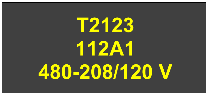
Figure 19. Transformer plate/label; 7/8-inch-high yellow letters on 4-inch high by 9-inch-wide black background (figure is approximately 1/2 scale). I&O is responsible for labeling high-voltage transformers (TH).
