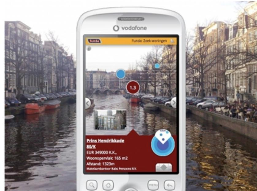
A camera phone with GPS processes images to recognize buildings and landmarks and provides relevant data from internet
