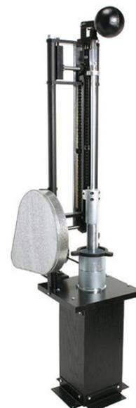
Figure 4.1.1: Compaction hammer
