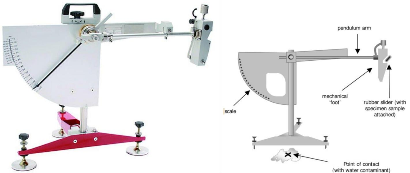
Figure 5.3.1: British pendulum tester
