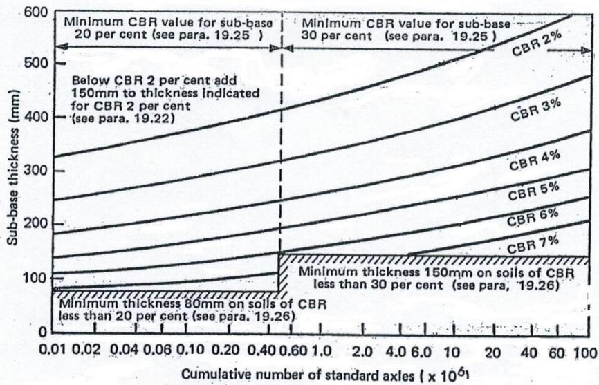
Fig. 19.9. Thickness of sub-base.
