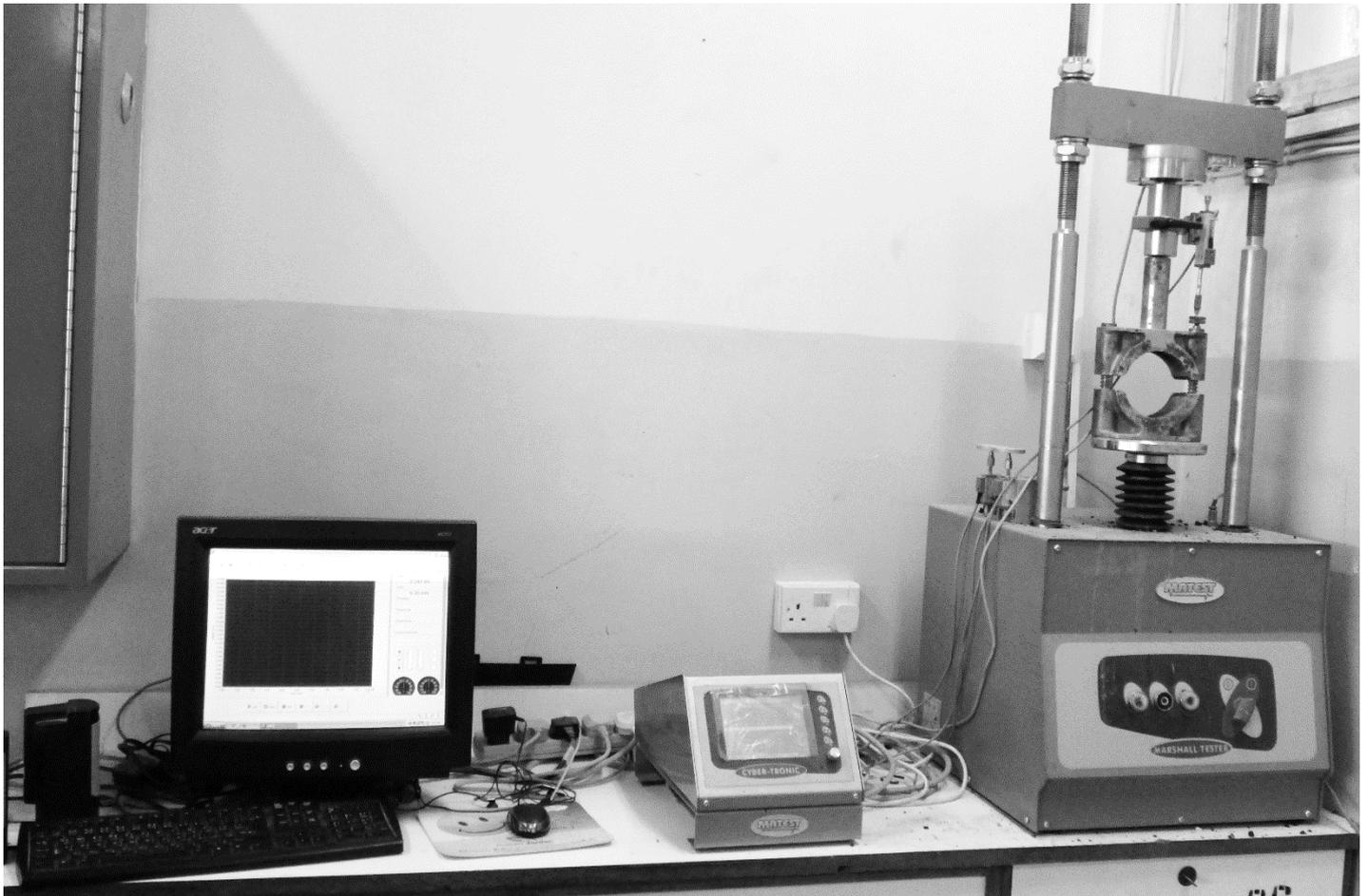
Figure 4.1.3: Marshall Apparatus
