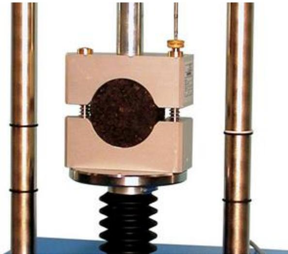
Figure 4.1.2: Breaking head
