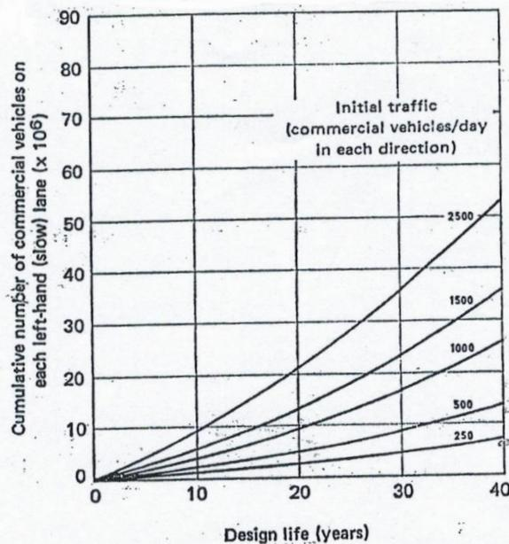
Fig. 19.4. Relationship between cumulative number of commercial vehicles carried by each left-hand (slow) lane and design life; growth rate 3 per cent.
