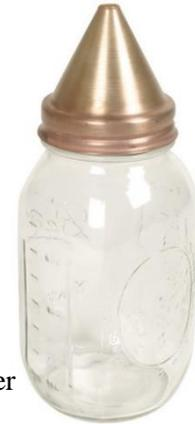
Figure 3.3.1: Glass Pycnometer
