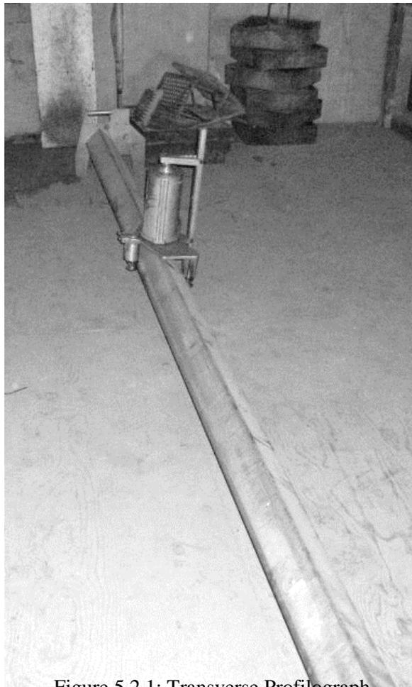
Figure 5.2.1: Transverse Profilograph
