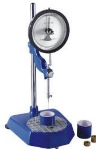
Figure 3.1.1: Penetrometer
