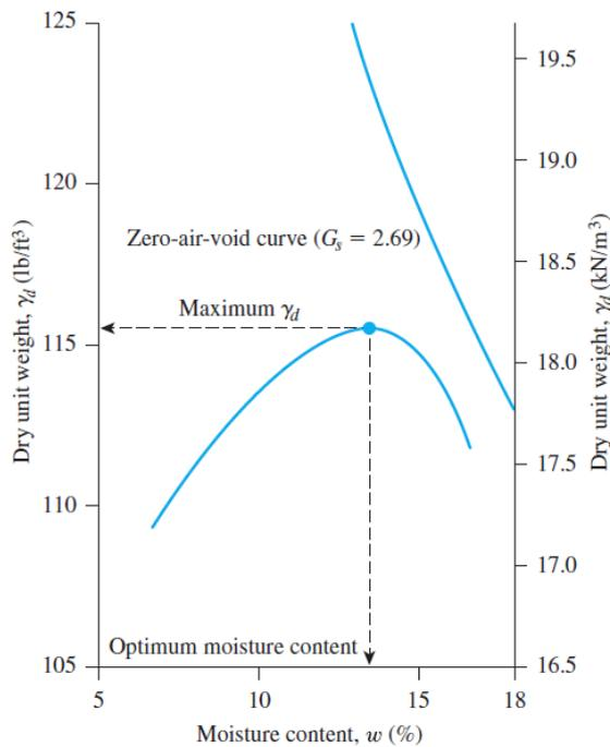
Figure 1.1.2: Moisture content with Dry unit weight
