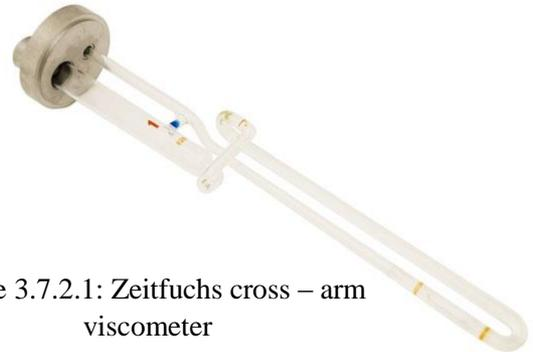
Figure 3.7.2.1: Zeitfuchs cross – arm viscometer
