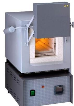
Figure 5.1.1: Oven / Muffle furnace
