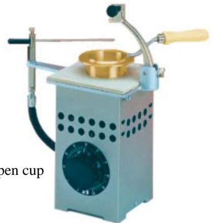
Figure 3.5.1: Cleveland open cup apparatus
