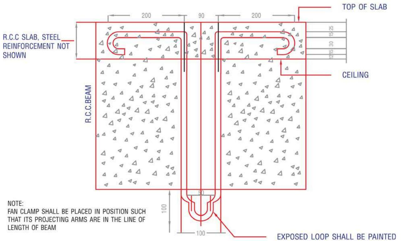
TYPE 2 WHERE FAN CLAMP IS TO BE FIXED DURING LAYING OF R.C.C. BEAM
