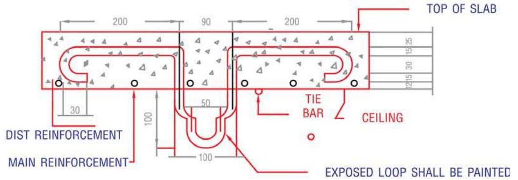
TYPE 1 WHERE FAN CLAMP IS TO BE FIXED DURING LAYING OF R.C.C. SLAB
