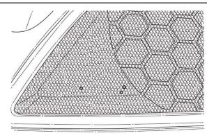
32. Remove masking on the backside of the badge. Position badge onto door panel using the two holes widest apart.
