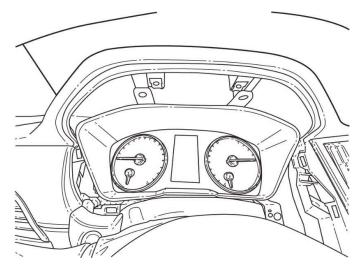
7. Dislodge (27) clips to carefully remove the upper dash panel. Start at the right side and work towards the radio.
