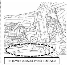
15. Route accessory amplifier harness blue and gray connectors towards underneath the passenger seat following the same path as the yellow-taped factory harness. Secure with (3) wire ties at the white tape mark locations to the factory harnesses wrapped in black tape only. Do not secure accessory harness to yellow factory harness. Continued...
