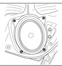
30. Install new speaker using factory hardware and reconnect harness.
