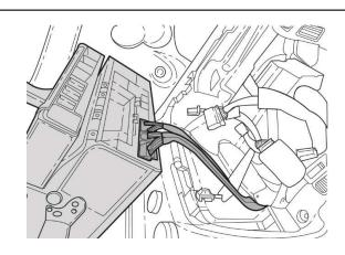
22. If CD player was not installed, secure the CD player extension harness to the side of the console box. Fold the harness in half and use (1) wire tie at the white tape mark to secure the harness to the RH side of the console box. Wrap the white connector to the foam harness using (1) piece of included 70x100mm foam tape as shown.
