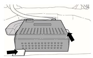
19. Wrap seat harness with (2) pieces of included 70x100mm foam tape. Ensure harness covers the area that touches the amplifier bracket. This is to prevent noise and rattles.
