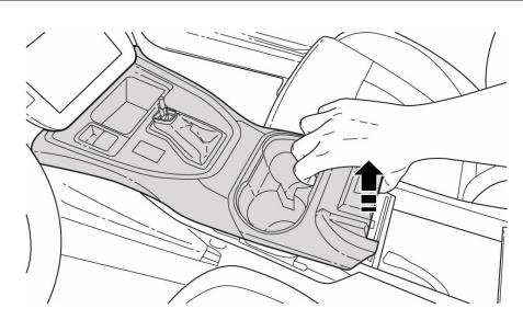
11. Unplug the white connector under the center console panel and remove from the vehicle.
