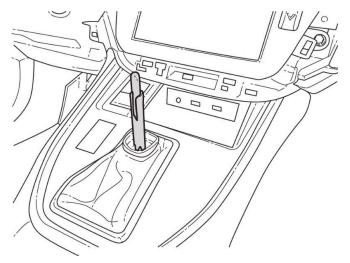
10. Remove the upper center console panel by grasping near the cupholder and firmly pulling upward.
