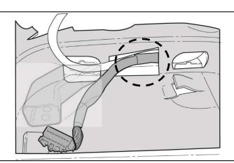
18. Place amplifier under seat aligning bracket with two threaded studs found under two relief cuts in carpet. Connect harness to amplifier. Secure with two included nuts torqued to 7.5 N/m (+/-2) as shown.
