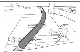
20. Make connections at radio location. Connect the accessory harness 6-pin and 10-pin connector ends that are wrapped in foam to the two vehicle harness radio connectors. Connect the 4-pin accessory harness connector to the vehicle prearranged 4-pin connector secured to the OEM Harness with pink breakaway tape.
