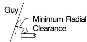
**Figure 2 Radial Clearance**
