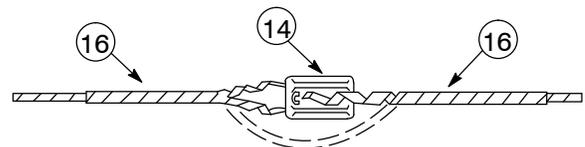
When "shorting-out" insulator (as required in Case 1 on Page 3), install the guy wire in one continuous piece as shown by dashed lines.
