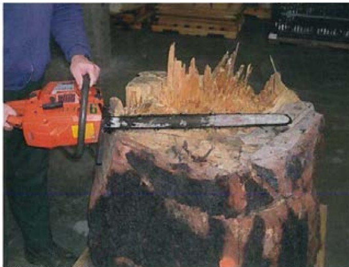
Photo 3 Stump of Tree 1 with saw illustrating multiple gunning cuts.
