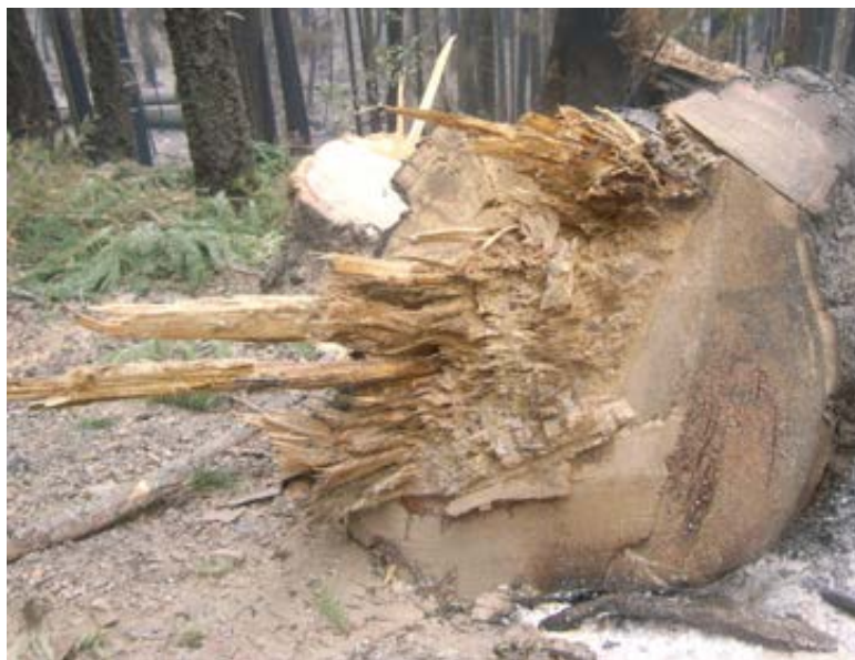
Photo 6 Butt section of Tree 1 showing excessive holding wood, two gunning cuts and Dutchmen
